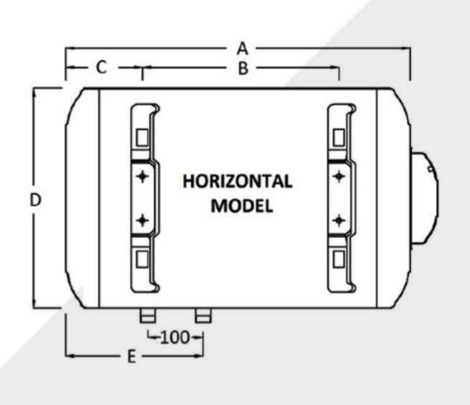
Max. Working Pressure: 0.8MPa Rated Voltage: 220-240VAC, 1 Phase
